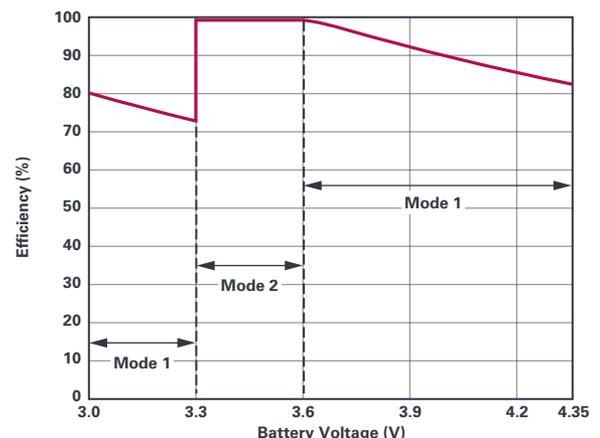
Figure 2. Theoretical maximum converter efficiency vs. battery voltage.
