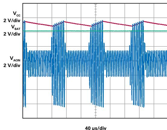
Figure 1. Rectification of ac input and regulation of dc rail voltage.
