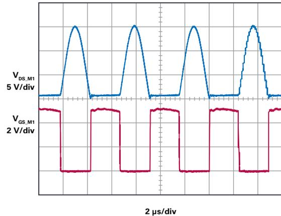
Figure 5. ZVS operation when  $f_{TX\_TANK} = 1.29 \times f_{DRIVE}$ .
