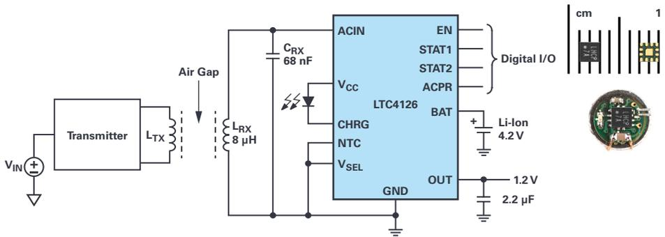
Figure 3. Complete 6 mm diameter wireless battery charger receiver with integrated dc-to-dc converter and charger status outputs.
