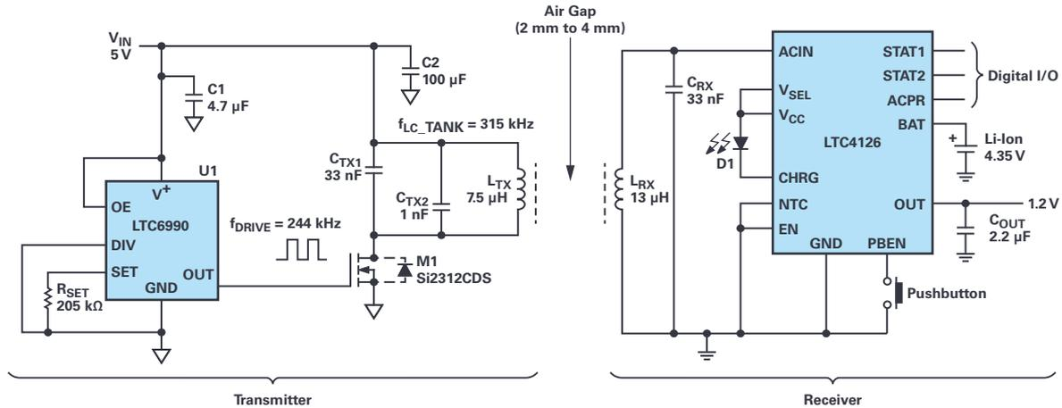
Figure 4. Complete wireless charging solution with single transistor ZVS transmitter and the LTC4126 receiver.
